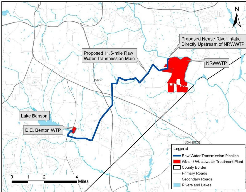
**Figure 3.5 - Neuse River Intake Above the NRWWTP**
