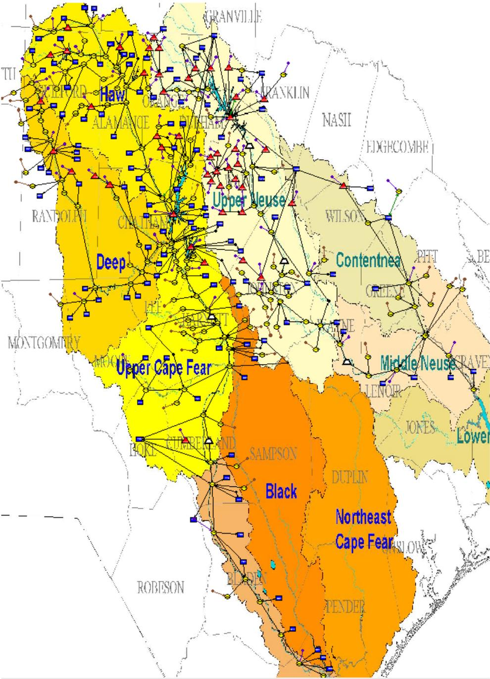
The user can click on any node or connecting arc on the schematic to access specific information, like reservoir elevation-storage-area data or minimum streamflow requirements. These data are also contained in tables contained on other tabs of the model.
