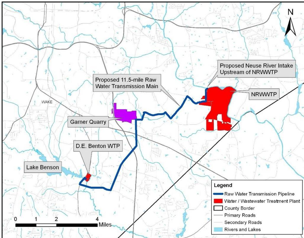
**Figure 3.7 - Neuse River Intake Above the NRWWT with Offline Storage**
